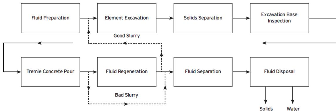
Figure 33. Support Fluid Lifeline During the Construction Process
