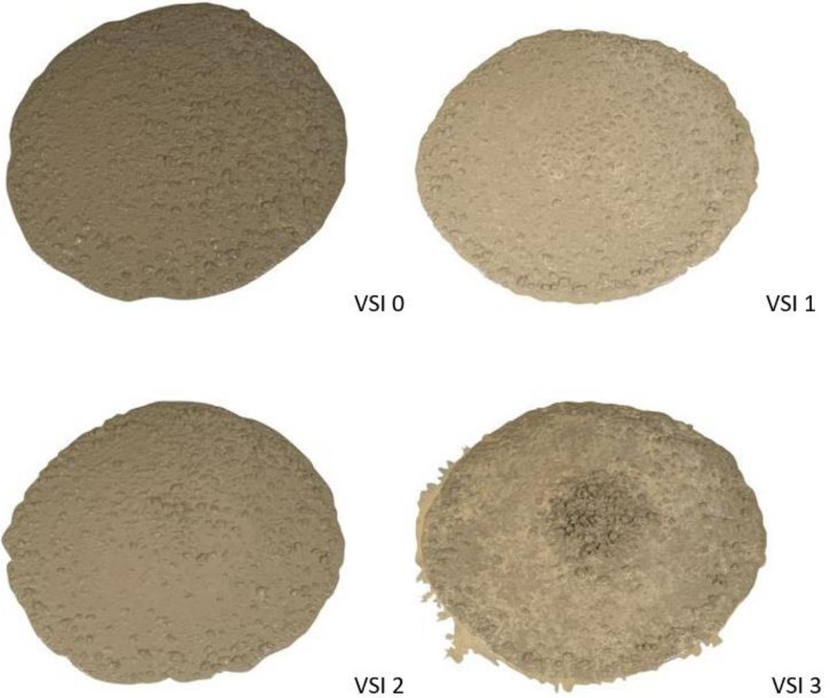
*Figure 29. Examples of Visual Stability Index Classes [1], photo courtesy of BASF Corporation*
