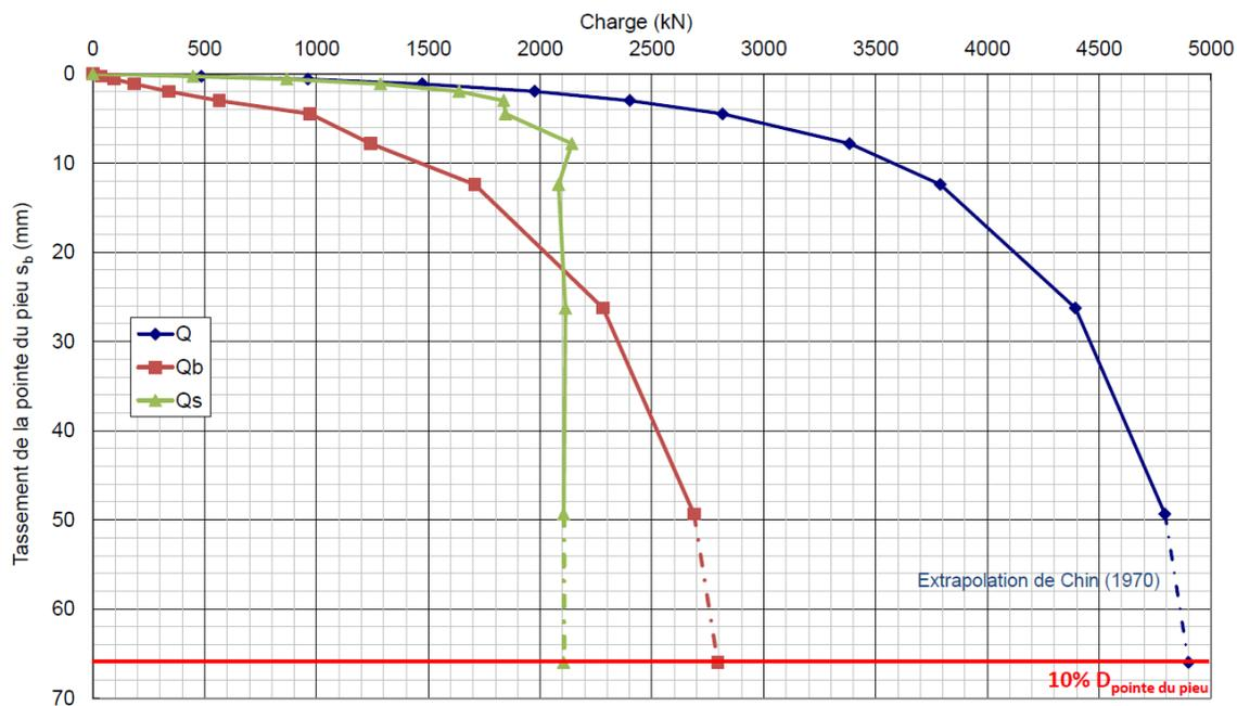
Figure 16. Haren test site - Load-settlement split up in pile base and shaft resistance
