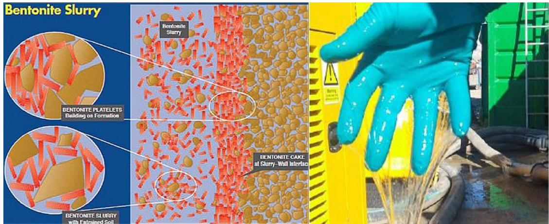
Figure 31. Comparative behaviours of bentonite and polymers
