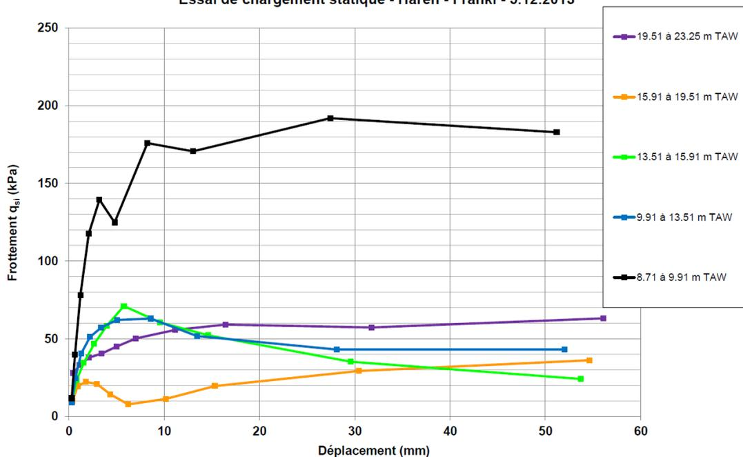
Figure 17. Haren test site - Mobilisation curves of the unit shaft friction in the relevant soil layers
