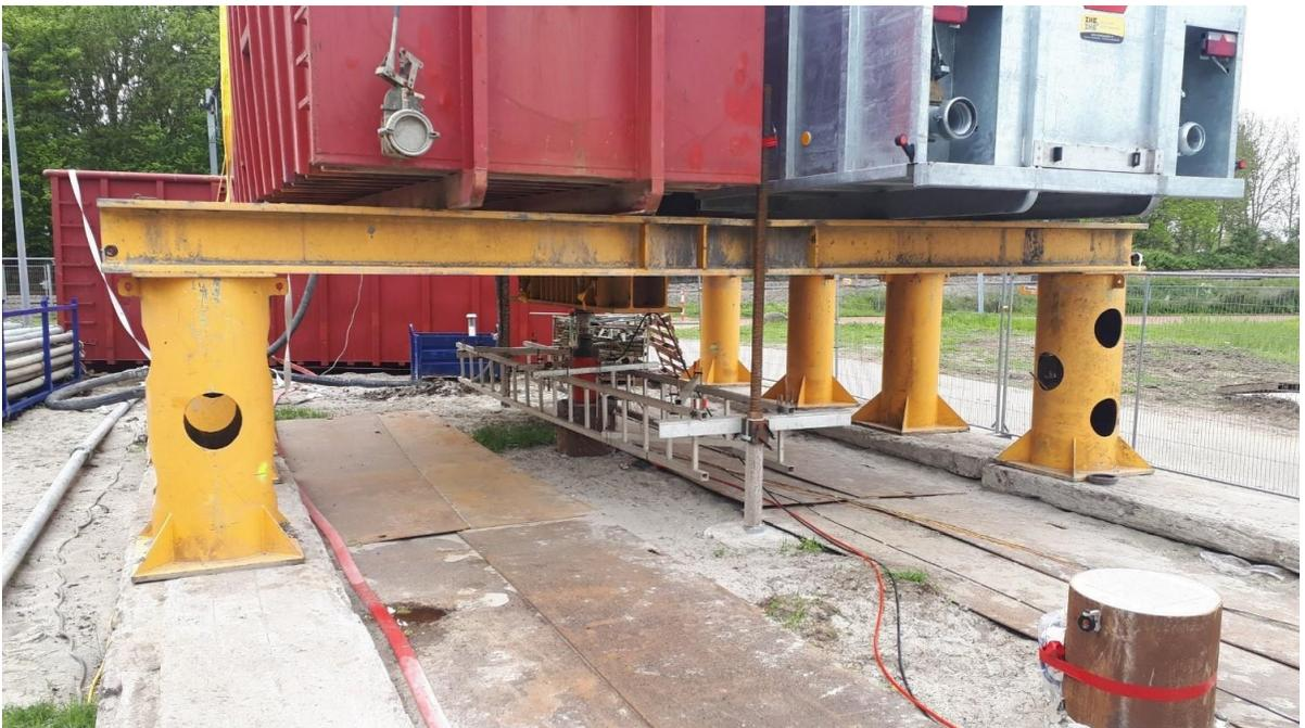
Figure 23. Set up of the compressive load test on a micropile
